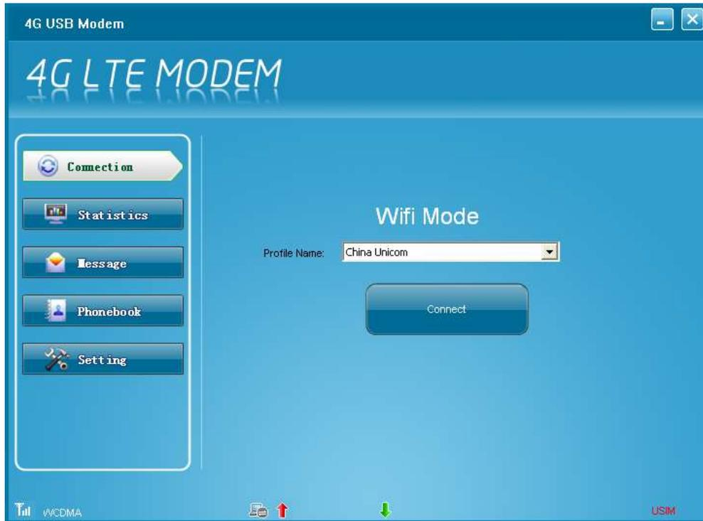
Figure 4-6 Connect 4G/3G Network
